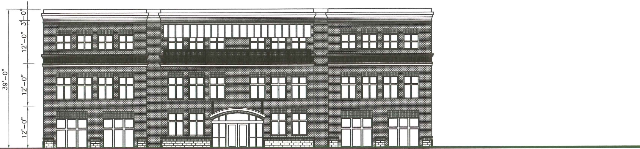
1 WEST ELEVATION (CALHOUN STATION PARKWAY) SCALE 1/8"=1'-0"
