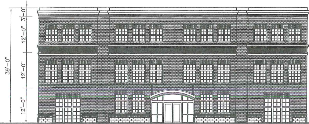
1 WEST ELEVATION (CALHOUN STATION PARKWAY) SCALE 1/8"=1'-0"
